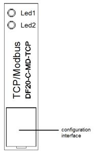
Set the configuration interface to facilitate the adapter program upgrade.
