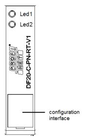
Set the configuration interface to facilitate the adapter program upgrade.
