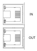
Used to establish communication with the upper computer. The coupler features an integrated 2-port switch, allowing easy line structure creation without additional network components.
